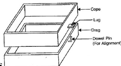
**Fig: Molding Boxes**
