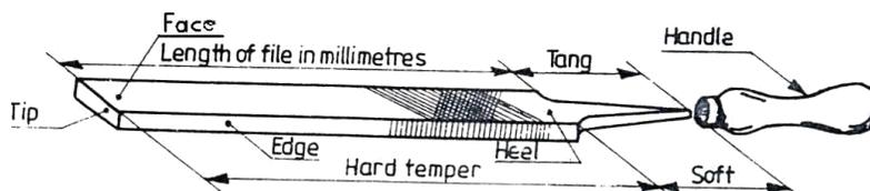
**Fig: Parts of a Hand File**
