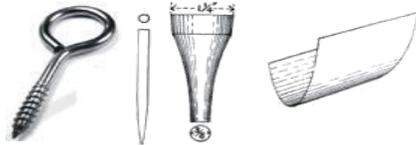
**Fig: Gate Cutters**
