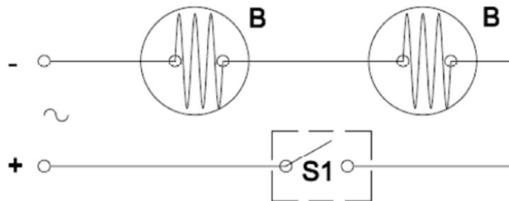
**TWO LIGHTS CONTROLLED BY ONE SWITCH IN SERIES**
