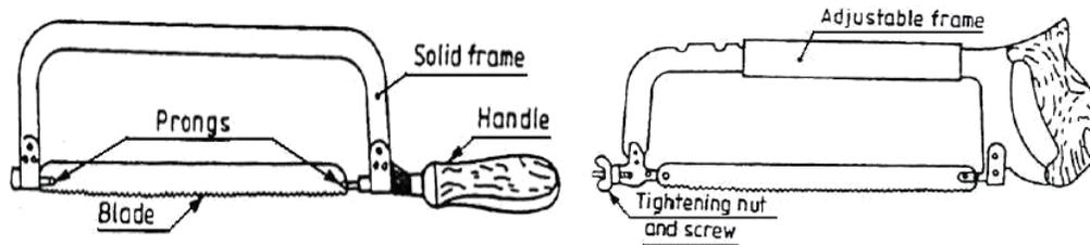
**Fig: Hacksaw Frame with Blade**
