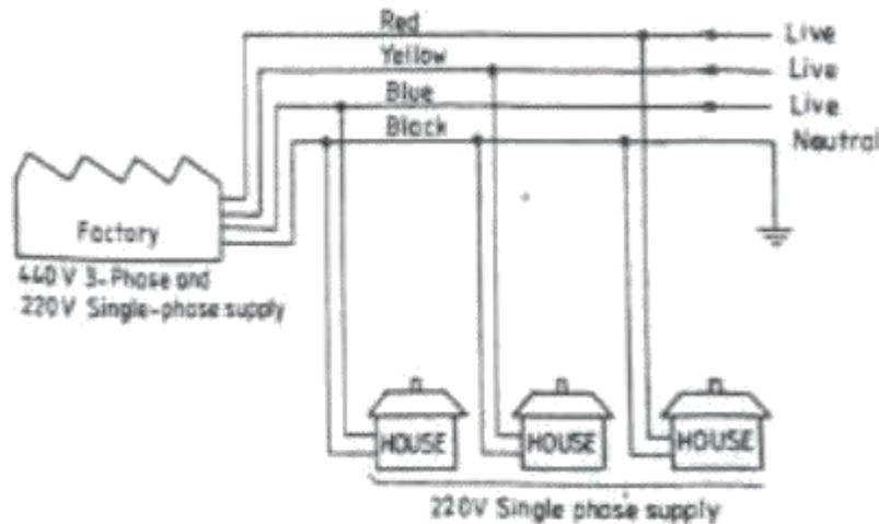
**Fig: 3 Phase – 4 Wire Supply**
