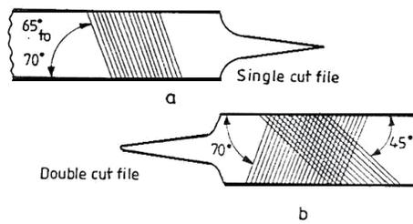
**Fig: Single and Double Cut Files**
