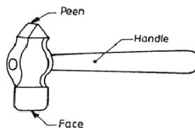
**Fig: Cross Peen Hammer**
