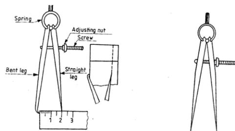
**Fig: Odd Leg Caliper and Divider**
