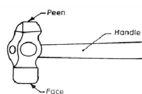
**Fig: Straight Peen Hammer**
