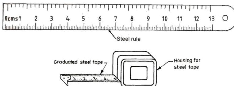
**Fig: Steel Rule and Steel Tape**
