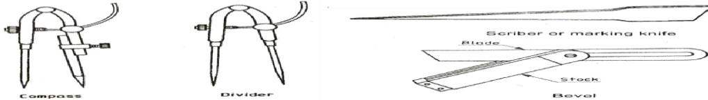
**Fig: Compass and Divider**
