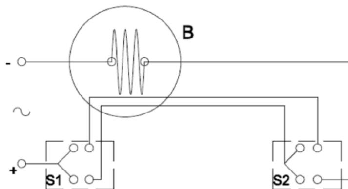
ONE LIGHT CONTROLLED BY 2 TWO -WAY SWITCHES
