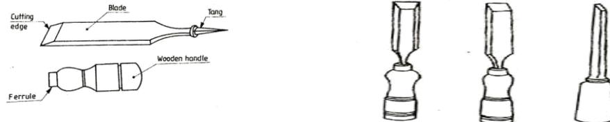
**Fig: Types of Chisels**
